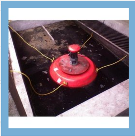
High Speed Floating Aerator
